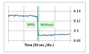
Figure 9: Power Fator with and without SinuMEC
