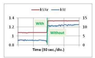
Figure 4: kW and kVAr during no load
