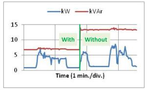
Figure 3: kW and kVAr with and without SinuMEC
