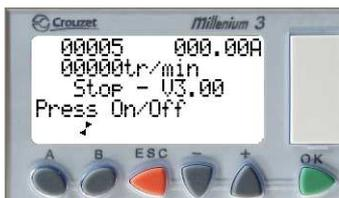
If this error occurs three times on the same open or close cycle, the display shown on the adjacent figure will blink.
