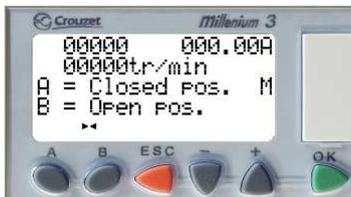
**Programming the limit positions "open" and closed".**
