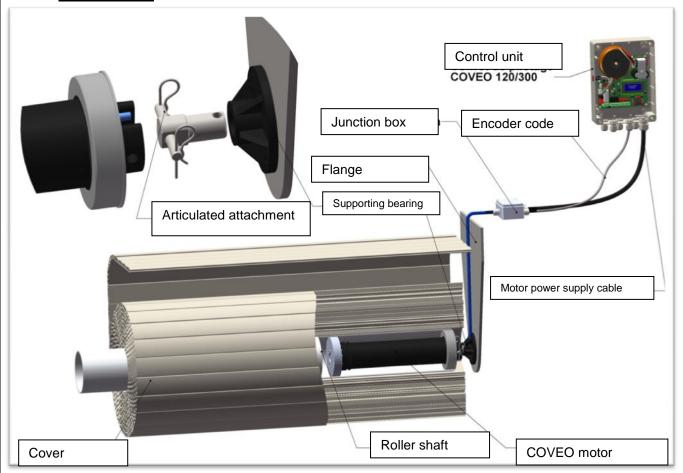
The force applied to the motor is taken up on the fixed shaft by the customer's supporting bearing (no dual articulation).
