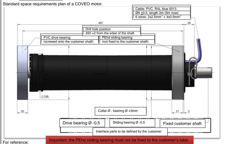
the fixed shaft that links the motor to the supporting bearing and the diameter and shape of the bearings may vary according to the customer's requirements. Each motor has a detailed space requirements drawing, validated by the customer.
