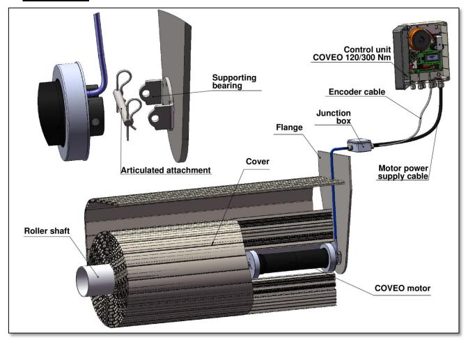
The force applied to the motor is taken up on the fixed shaft by the customer's supporting bearing (no dual articulation).
