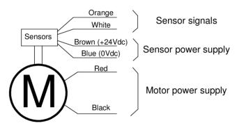
Connection in a waterproof junction box filled with gel or resin is compulsory.
