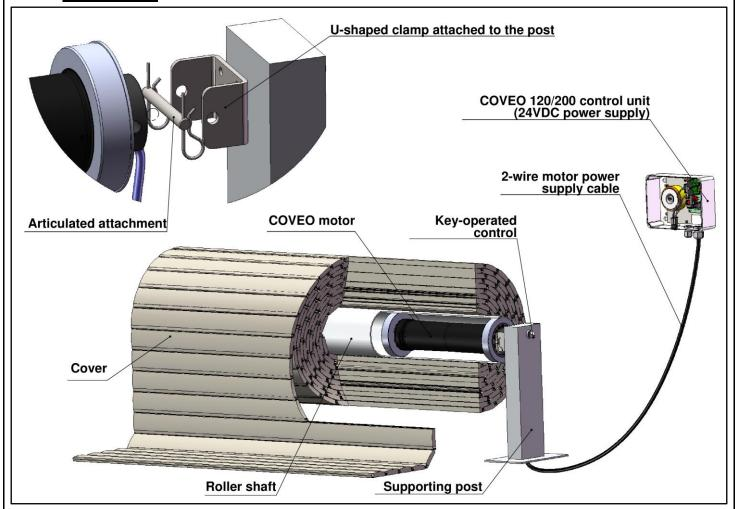
The force applied to the motor is taken up on the U-shaped flange by the supporting post (no dual articulation).
