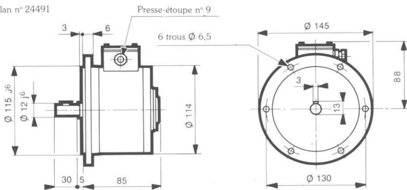
This alternator delivers a single phase e.m.f. whose distortion rate is less than 3 %. The standard electrical characteristics are indicated in the table below.
